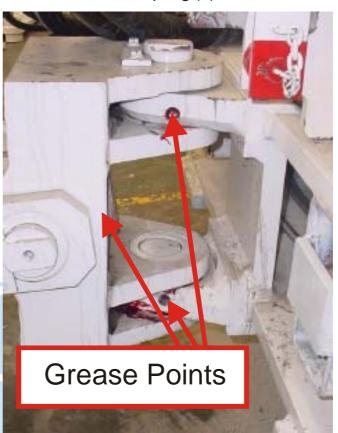
Swing Arm Hinge Pins (4) Swing Arm Guide Plate (10)
