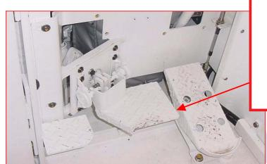
Brakes dump to ZERO automatically when engine shuts down. If they fail to dump, the machine is FAULTY and must NOT be used until faults are rectified.
