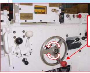
Drain Steering Accumulator by steering back and forth until Accumulator Gauge reads ZERO, or release Accumulator Dump Valve.
