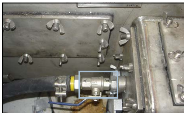
Wet Bath Exhaust Conditioner - Main Supply/Isolation Valve
