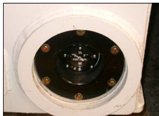
Fuel Tank Inspection Cover Drain Plug Underneath
