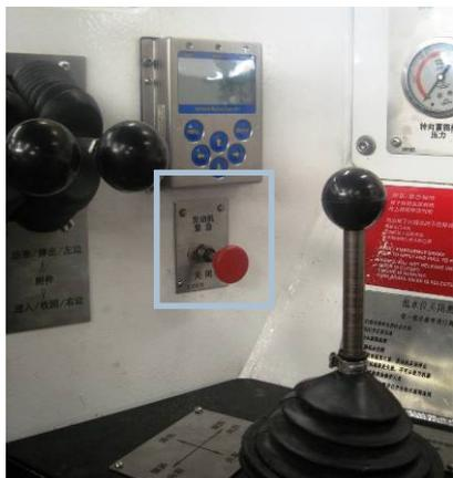
紧急进气关断阀—关断按钮
